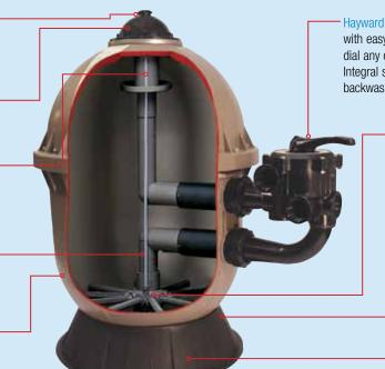
Hayward 7-Position Vari-Flo Control Valve with easy-to-use lever-action handle lets you dial any of the seven valve/filter functions. Integral sight glass lets you see when backwash cycle is completed.
